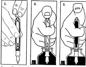
1 Remove Tip of barrel (by few turns to left) exposing Filler Button.
